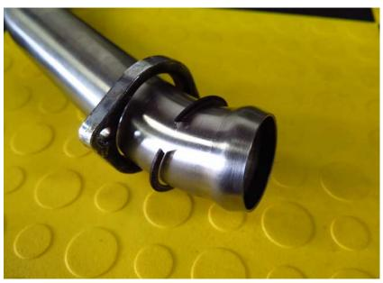
8. Begin by loosely installing the headers in the cylinder head and start the flange bolts, *don't tighten them yet*.
