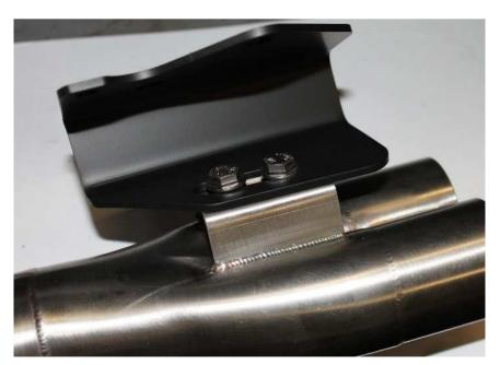
11. Test fit the collector to header BEFORE applying the high-temp sealant. Reattach brake rod first. Note the alignment of the bolt holes to engine case and make sure brake rod is inside the bracket. Once you've confirm fit, apply sealant and slide collector onto header tubes. *Don't install collector springs yet*.
