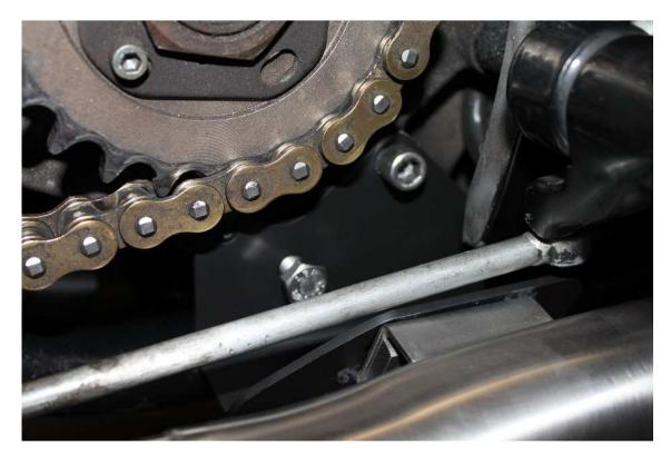
13. Tighten the bracket to the engine, and the bracket to the muffler. Checking frequently for proper alignment. *This is where you are going to make most of your adjustments to properly align the muffler relative to frame and swingarm.*
