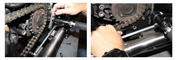
14. Once everything is aligned properly, then tighten the muffler support bracket in all locations. Tighten the cylinder head flanges to proper specification.
