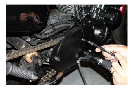
4. Remove muffler support bracket, either OEM/aftermarket as applies, from behind the side cover. Note location of the hardware removed and save, some bolts will be reused.
