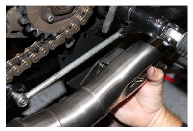
12. The frame bracket will attach to case using an original allen head bolt in the upper right corner of bracket. The lower, middle hole will use the hex head bolt provided in the kit (can't tighten allen head style bolt due to bracket clearance). The upper left side bolt hole will be filled when you install the side cover bolt (now is a good opportunity to make sure it has clearance for that bolt).
