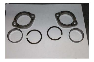
7. Transfer your existing cylinder head spring clips and flanges (or install new ones) onto the new exhaust. Make sure the indentation in the flange (for the spring clip to sit in) is facing in the proper direction.
