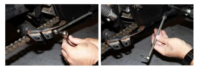
3. Remove primary drive side cover. Note locations of bolts and retain the hardware for reinstallation.
