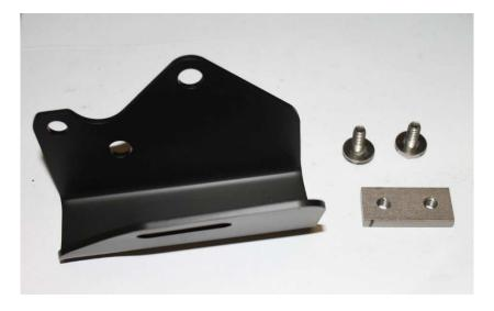
10. Attach the frame support bracket to the tab mounted on the exhaust with the provided hardware. Leave it loose so you have plenty of adjustment range.
